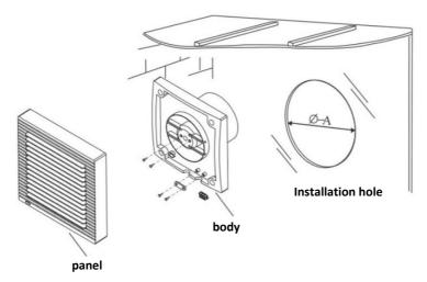
The product is equipped with two holes for power cable routing. A hole for the side power cable routing or a hole for hidden cable routing under the fan body.
